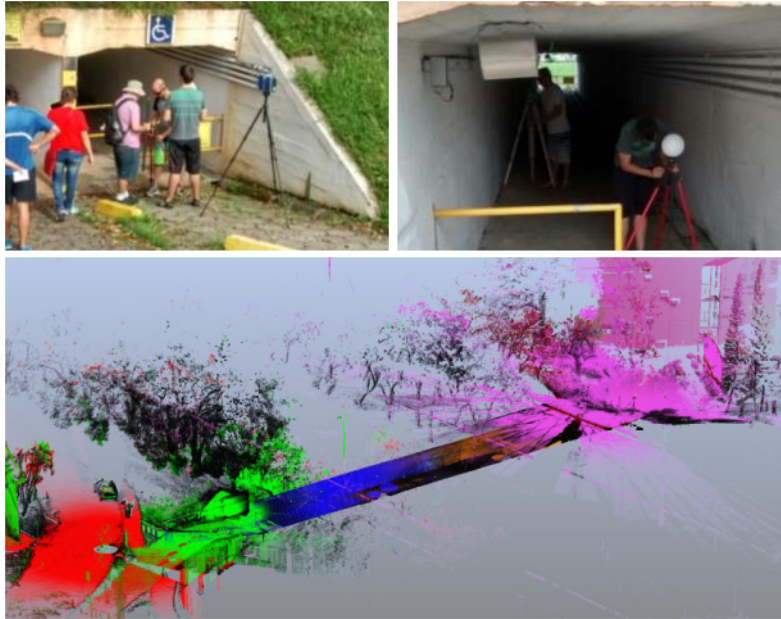
Figure 10. a) Laser scanner positioning in the tunnel entrance (above left); b) distribution of spherical targets inside the tunnel (top right); c) distribution of the six scenes in the survey of the underpass at UFSC (below)
