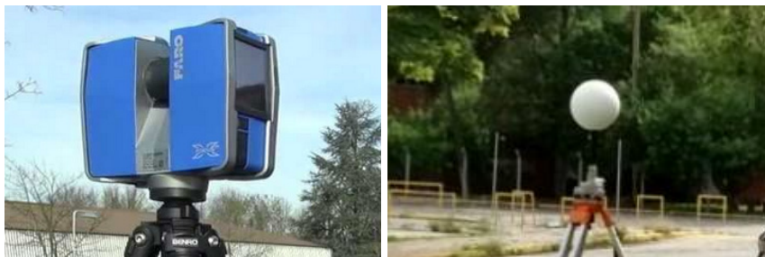
Figure 9. a) Terrestrial laser scanner Faro Focus3D x 330 (left) and b) spherical target positioned on the tripod with tribrach (right)
