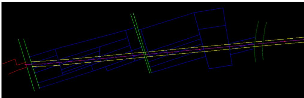
**Figure 9. Cadastral survey plan of power line (down) presentation of 3D restrictions due to servitude of passage (servitude is coloured in yellow, powerline centre line in purple, land parcel borders in blue and purple, and roads in green)**
