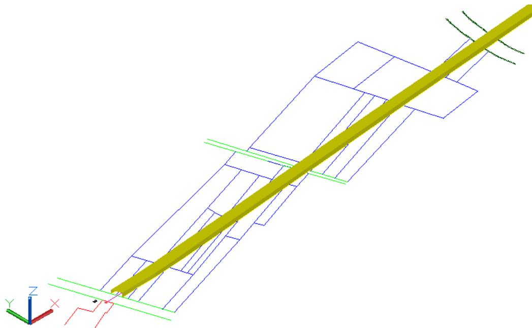
**Figure 10. Presentation of 3D restrictions due to servitude of passage (servitude is coloured in yellow, powerline centre line in purple, land parcel borders in blue and roads in green)**
