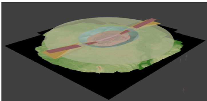
**Figure 4. 3D eTOD Obstruction Identification Surfaces in 3D pdf**
