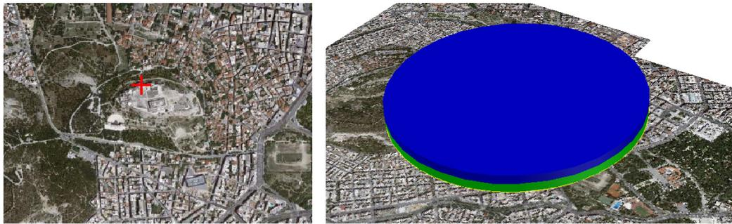
Figure 7. (left) Centre of no-flight zone in NCMA orthophoto (red cross), (right) No-flight 3D volumes in Autodesk AutoCAD software (no flight zone for propeller aircrafts is coloured in green while no flight zone for jets in blue)
