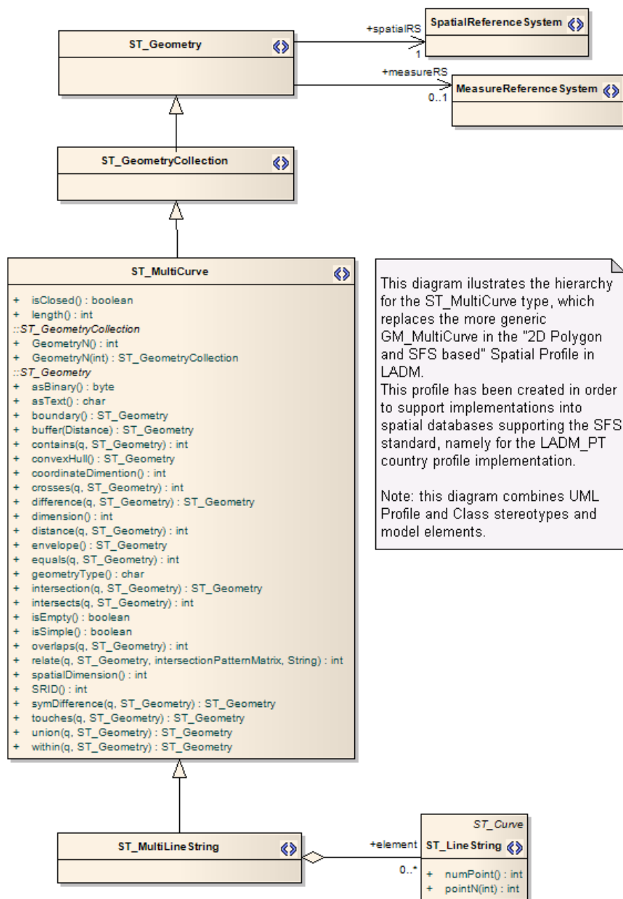
Figure B.1: Class (Profile) Diagram: The hierarchy of the SFS MultiCurve class
