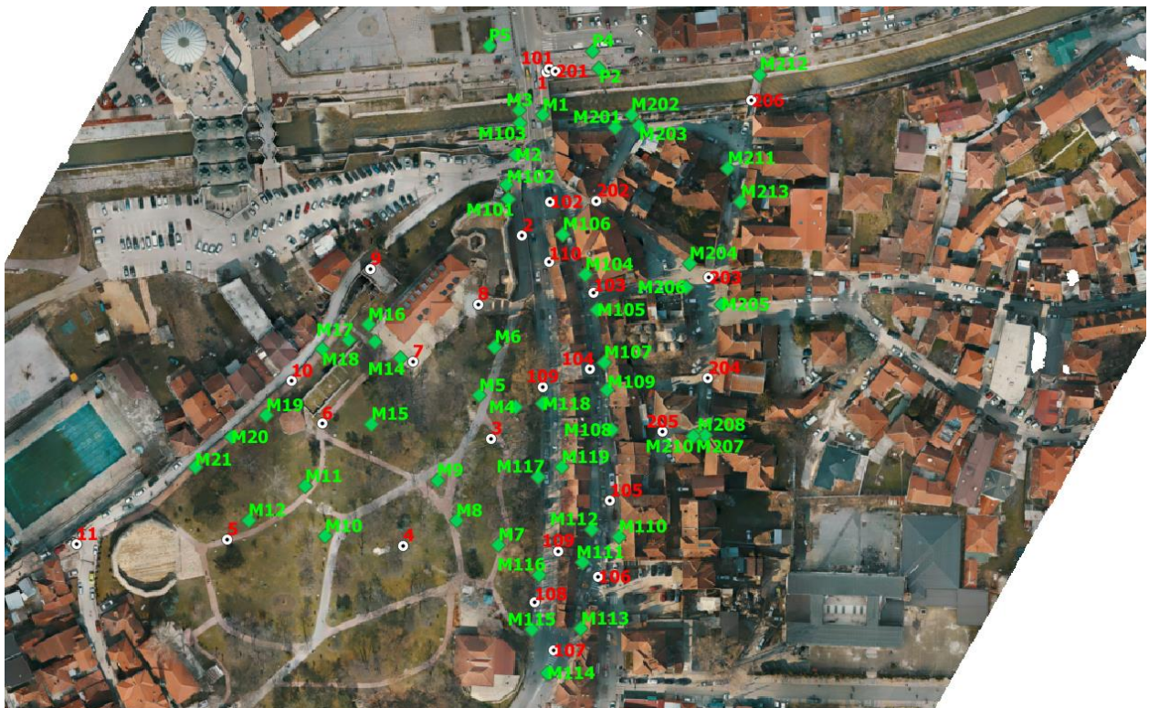
Figure 3. Scanning area. Stations are highlighted in red, marker positions are highlighted in green
