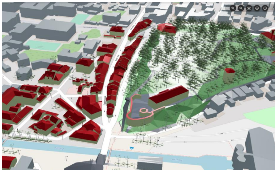
Figure 4. View of the 3D model with the corresponding features in Table 2 in accordance with the CityGML standard displayed in the Cesium JS Web Map Client – case study 2 – Novi Pazar
