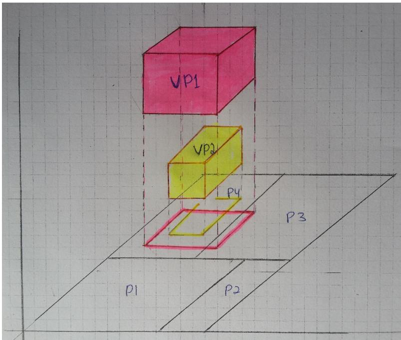
**Figure 4. VP1 and VP2 are 3D volumetric parcels overlaid onto the horizontal plane. The output is partial-overlap for VP1, and containment for VP2, where overlapping areas of both projected convex polygons are calculated by the Area function. Here, since VP1 and VP2 facades are planar, both convex polygons are constructed from points defining the X-Y plane**
