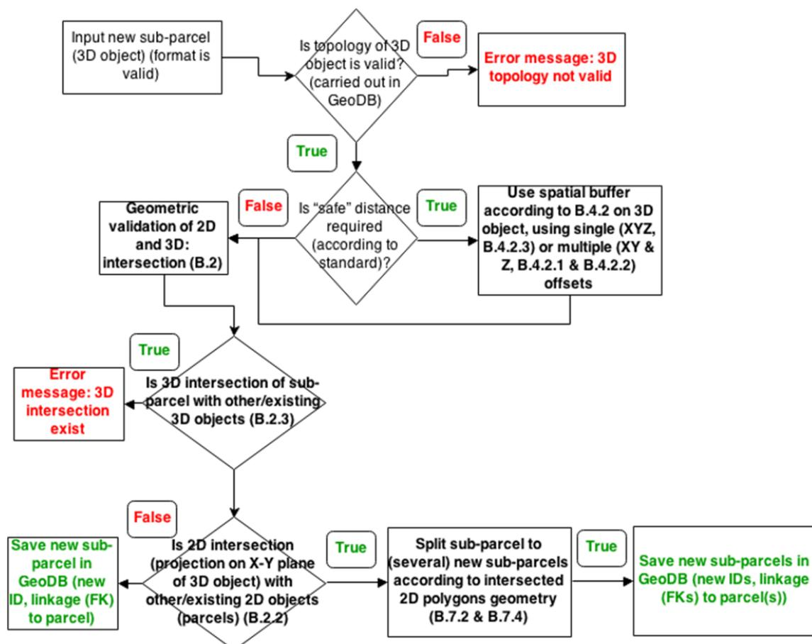
Figure 1. Insertion of a new 3D object (3D volumetric parcel, denoted here as sub-parcel) workflow
