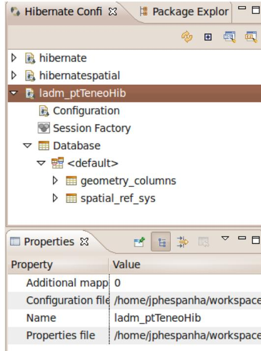
Figure 5.9: *Elements in an (empty) Hibernate Configuration*
