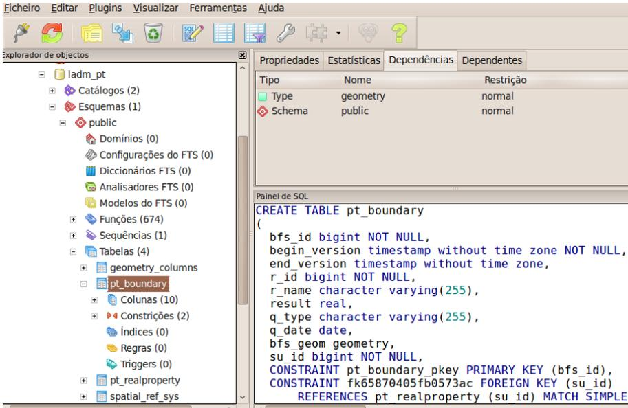
Figure 5.14: The *pt\_boundary* table details in PgAdmin III
