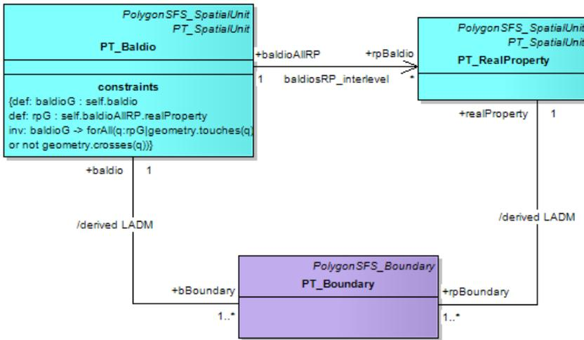
Figure 4.10: *Constraints between Real Property and Baldios*
