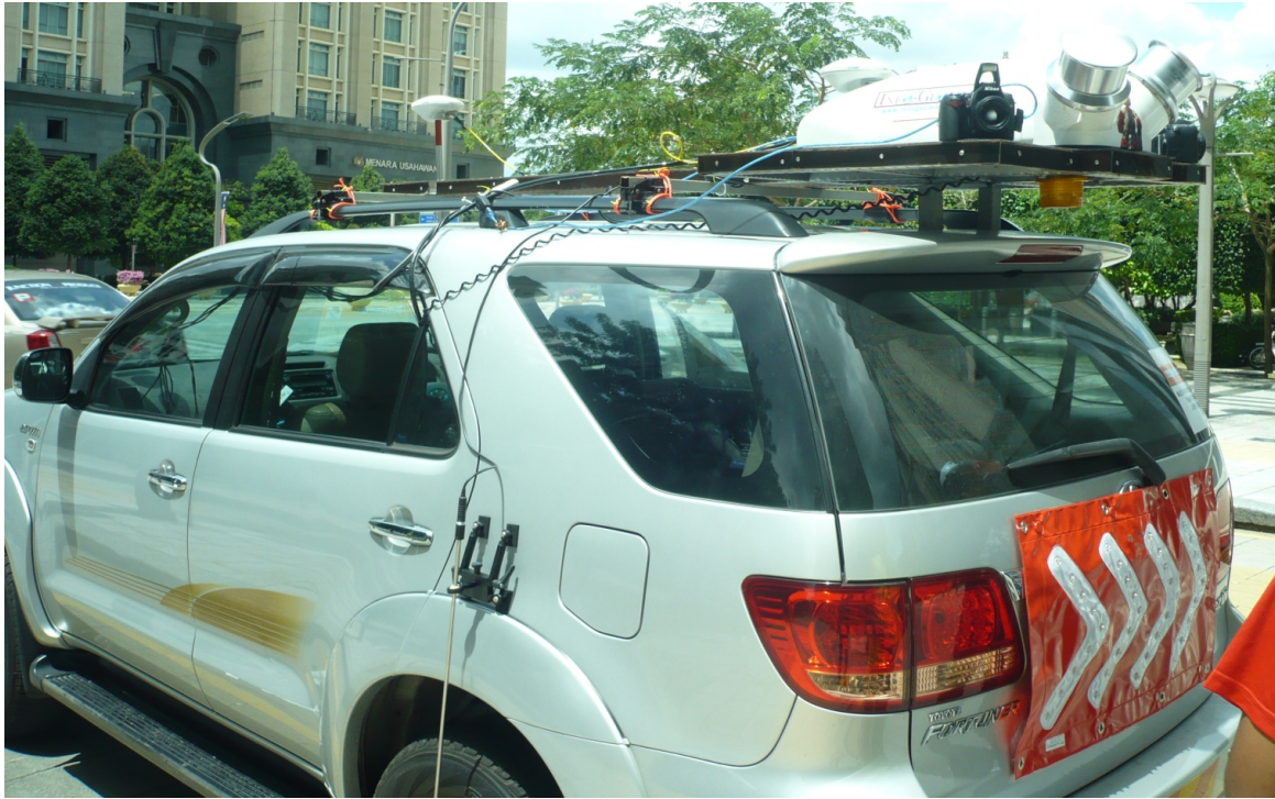
Figure 1: MTLS Dual Laser DynaScan 3 system used
